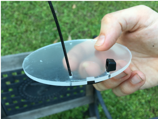
(b) First 3 mm acrylic layer showing how to thread the first cable tie
