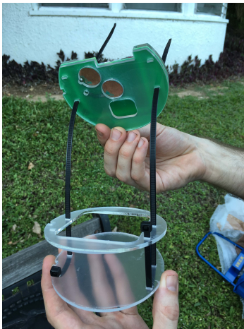
(d) Third 3 mm acrylic layer combined with PCB assembly
