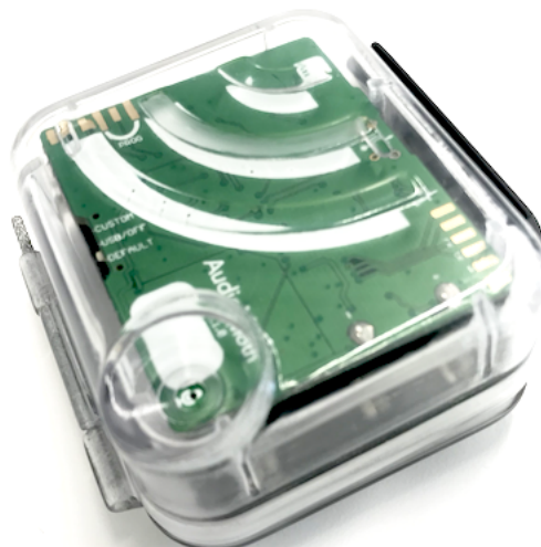
Figure 6.1: GoPro style enclosure to improve usability, durability and omni-directionality during outdoor deployments
