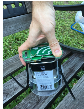
(f) Cable ties can be tightened during push force
