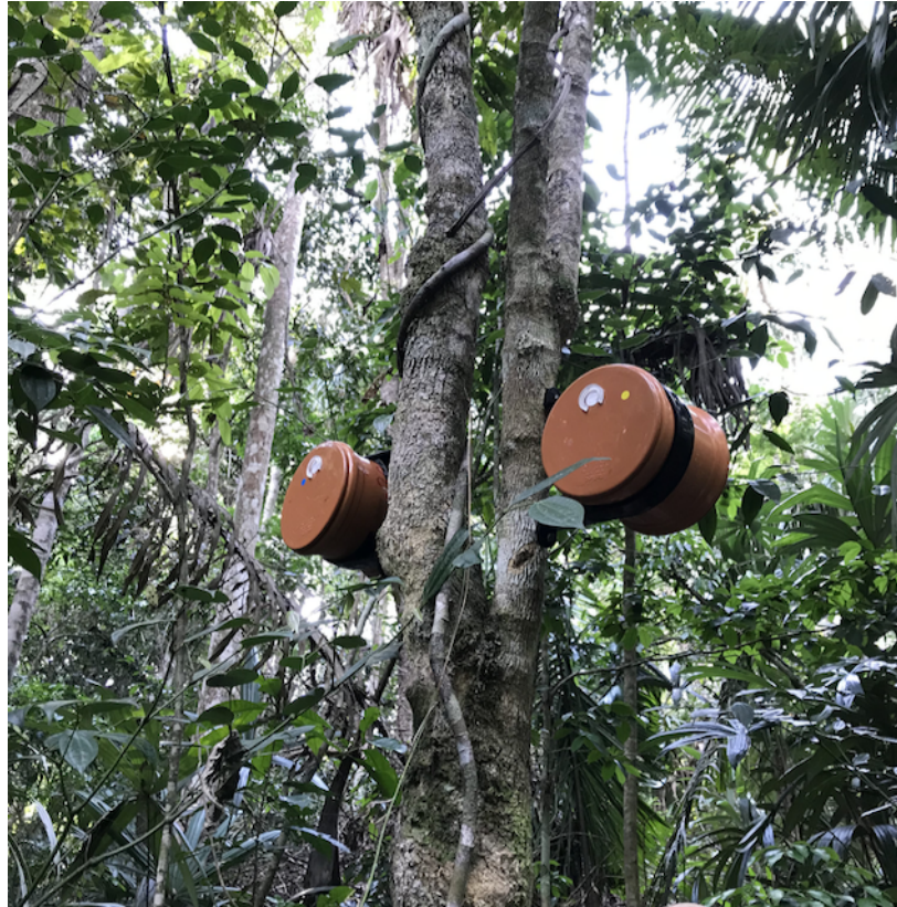
Figure 5.12: The 2018 AudioMoth gunshot algorithm deployment inside the 6 V enclosure
