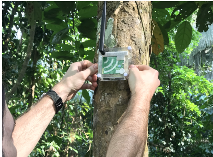
(b) LoPy extension module attached to AudioMoth GPIO ports, with a custom acrylic enclosure for LoRa gunshot alerts
