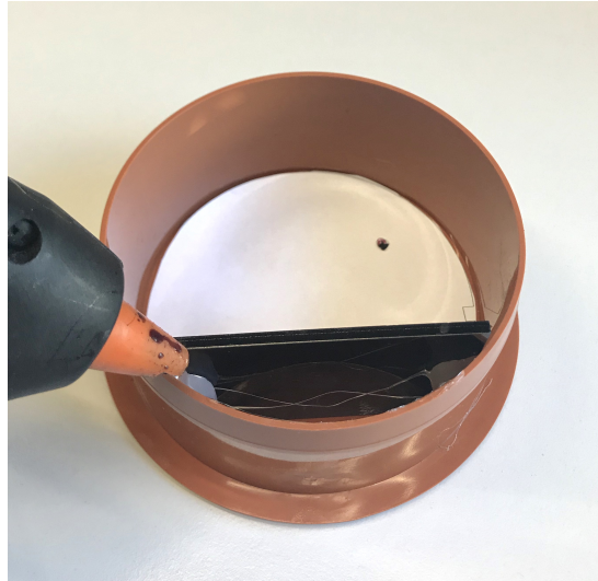
(b) Aligning drill hole and acrylic locking rectangle with printed jig
