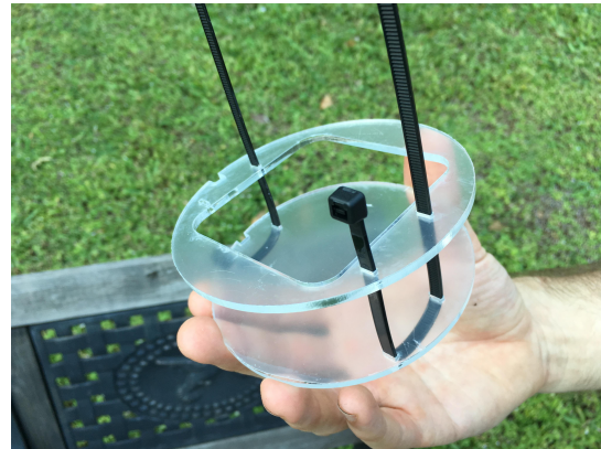
(c) Second 3 mm acrylic layer showing how to thread the second cable tie
