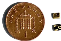
Figure 2.6: Illustrative figure demonstrating the size of MEMS microphones
