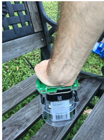
(e) Push force on top of PCB assembly to thread cable ties
