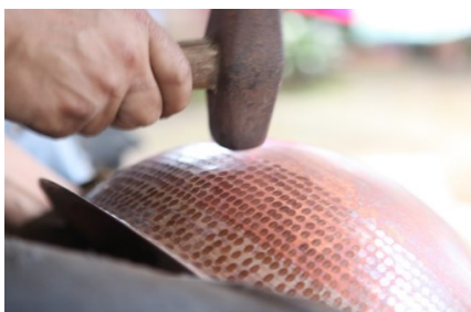
Figure 5.42 Hammering copper is a painstaking job requiring rythmical and armonious hammering, applying controlled force, with precision and dexterity. I noted Hernández's artisans do not count hammer blows. Santa Clara del Cobre, Michoacán. CADA Foundation®, November 2014.
