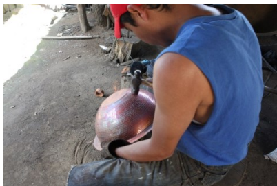
Figure 5.41 A young apprentice hammering a copper bowl by hand. Tools and hammers are build and created specifically for hammering special pieces. Santa Clara del Cobre, Michoacán. CADA Foundation®, November 2014.
