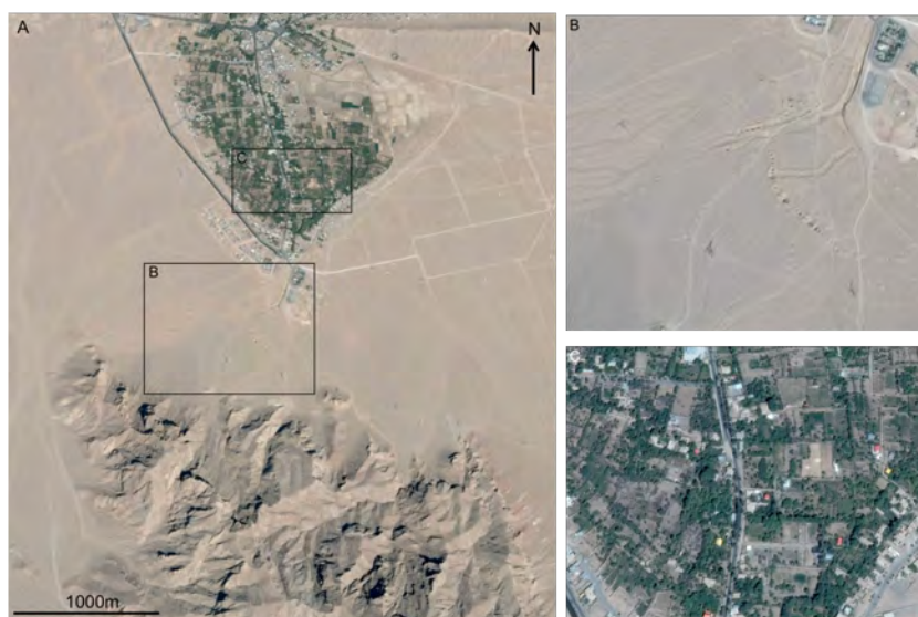
Figure 5.5: An example of a Qanat system, Joupar, South-east Iran. A: The hilly area to the South is the source area of the system. The village and irrigated fields are to the North. B: A number of spoil heaps outlining the path of the Qanat. C: The irrigated fields. Channel paths can be inferred by the linear features present. Images taken from Google Earth, May 2015.
