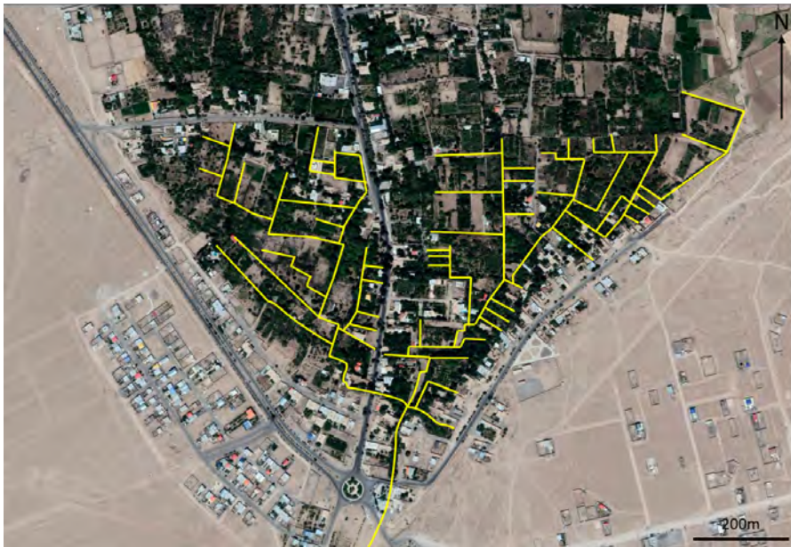
Figure 5.6: Top - Increased scale image of the Qanat system, Joupar. Bottom - Yellow : Interpretation of the Irrigation Network from Remote Sensing. Image taken from Google Earth, November 2019.
