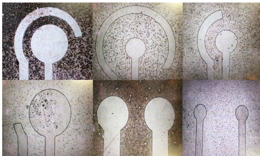
Figure 3.10: Photolithography pattern of Working and Counter electrodes.
