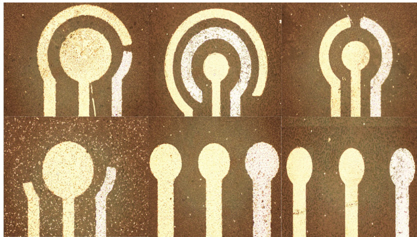
Figure 3.11: Fabrication of different sensor's designs.
