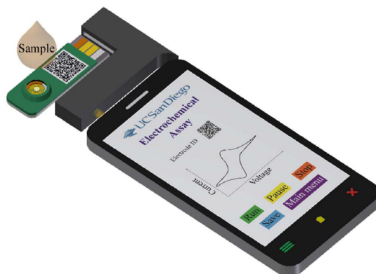
Figure 2.17: POC Electrochemical biosensor based on smartphone (79).
