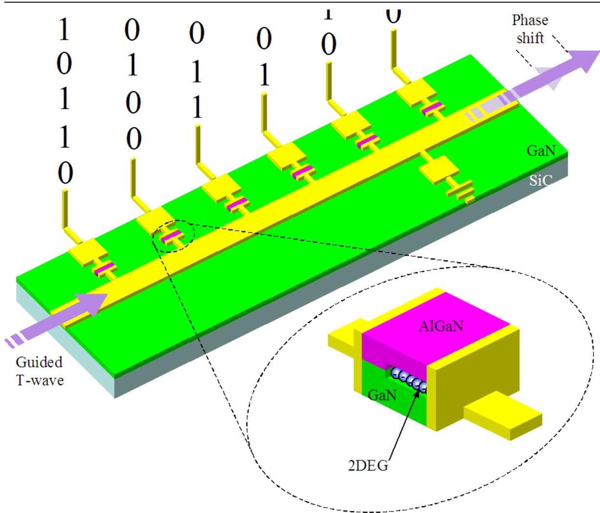
Figure 1. Schematic of the THz phase shifting chip and how it imparts digitally coded phase modulation to a T-wave, which is propagating along the central waveguide. The phase shift is introduced via the stubs that run along the upper side of the waveguide and act as tiny THz resonators controlled by micro-capacitors featuring a 2D electron gas.
