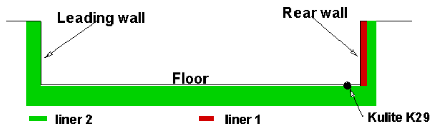
Figure 4.1: Liner positions in a 2-D cavity.
