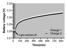
**Fig. 6.** Battery bank voltage during the charging phase. Charge 1 was during day 8 and charge 2 during day 9 (1 point every 2 min). Dark grey area indicates the period when the lights were on, prior being switched off (light grey area).
