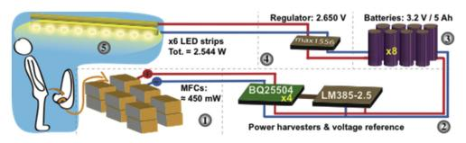
Fig. 2. Diagrammatic representation of the MFC system: the urinal feed the MFC stack (stage 1), from which the energy is harvested (stage 2), at a constant voltage by 4 power harvesters connected in parallel, and stored in 8 parallel Lithium Iron Phosphate cylindrical cells (stage 3), connected to a voltage regulator (stage 4) connected to 6 LED strips lighting the urinal  $\approx$ 9h30 per day (stage 5).
