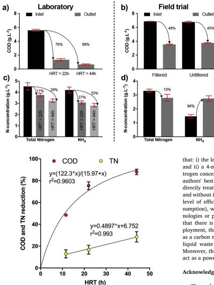
Fig. 7. Chemical Oxygen Demand (COD) (a, b), total nitrogen and ammonium reduction (c, d) in treated urine stream during laboratory investigation (a, c) and during the field trial at 11h40 HRT (**b. d**). The HRTs in (**a**) were obtained by changing the pulse-feed duty cycles: 22 h and 44 h correspond to 1.7L.2 h<sup>-1</sup> and 1.7L.4 h<sup>-1</sup>, respectively (Fig. 3).
