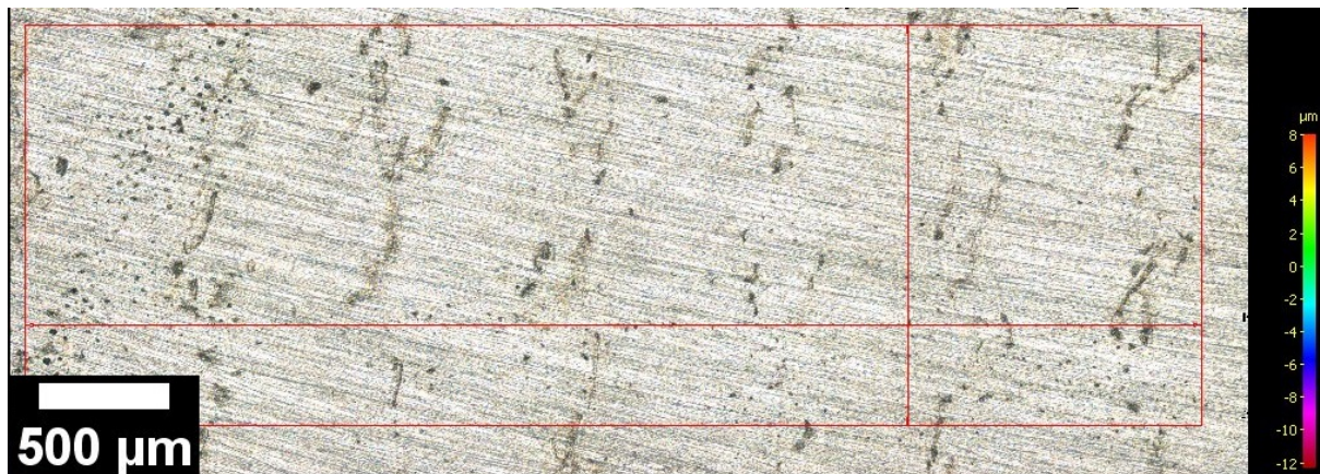
Figure 3-21 – LSP surface macro-image showing peening-generated pits may be aligned with ablative layer edges.
