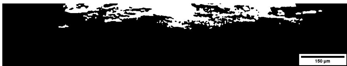
Figure 7-11 – Typical slice of segmented LSP pits.
