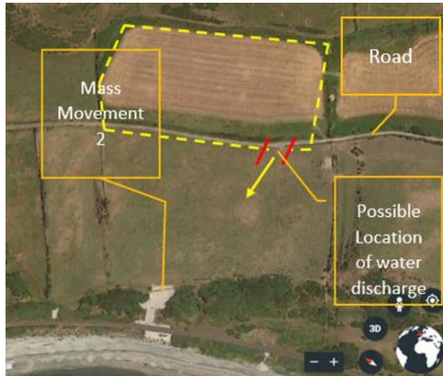
Figure 9-15 Discharge of water from the road at St Bees
