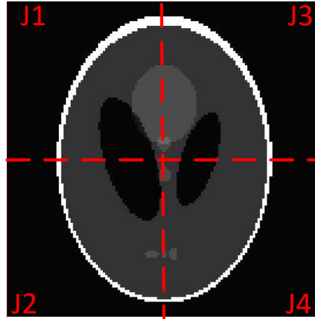
Figure 5.7: Partition the image into N = 4 blocks. If each block get de-noised separately, then the inner margins will be ignored due to the definitions of TV norm, thus affecting the approximation of the TV de-noising on the whole image. “inner margins” here refer to the boundaries between neighbouring sub-image blocks. For example, the inner margins of image block \mathbf{x}_{J_1} are the right and bottom margins.
