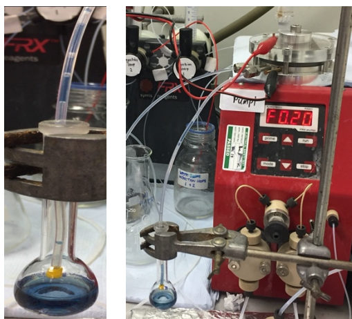
Figure 2.4: Pictures illustrating slug flow from the Ammonite 8 reactor
