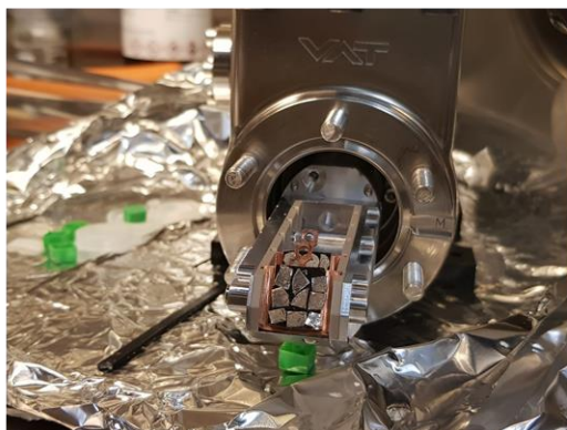
Figure 2.33 – (a), Front and (b), side-view of samples loaded into the vacuum suitcase.
