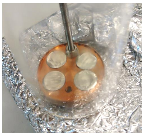
Figure 4.5 – Battery-grade lithium foil inside the portable reaction vessel before (a), and after (b), 2 hours nitridation.
