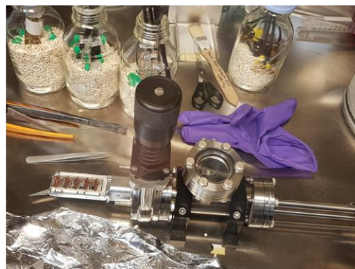
Figure 2.33 – (a), Front and (b), side-view of samples loaded into the vacuum suitcase.
