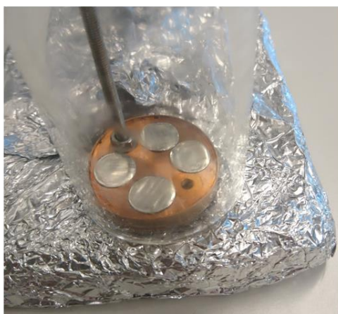
Figure 4.5 – Battery-grade lithium foil inside the portable reaction vessel before (a), and after (b), 2 hours nitridation.
