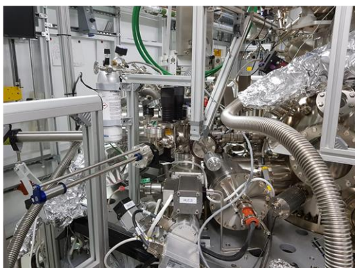
Figure 2.34 - (a), Sample transfer suitcase mounted onto the I09 end-station. The suitcase is opened to ultra-high vacuum prior to inserting the sample into the instrument. (b), I09 end-station.
