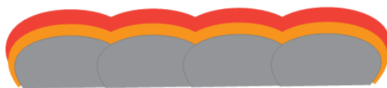
Figure 4.26 – Schematic illustration for the formation of a thick SEI layer on lithium metal electrodes.
