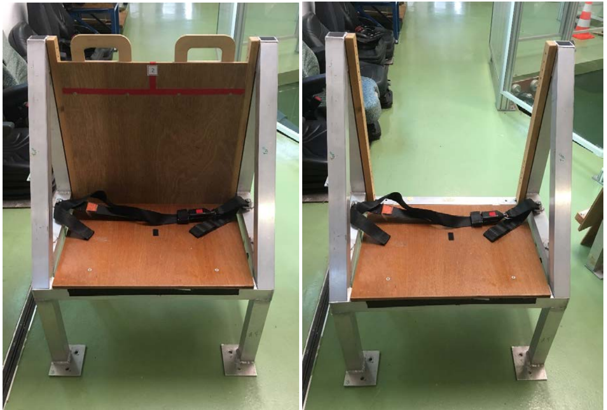
Figure 3.4 Rigid seat used in experiment 1 with and without the backrest present.
