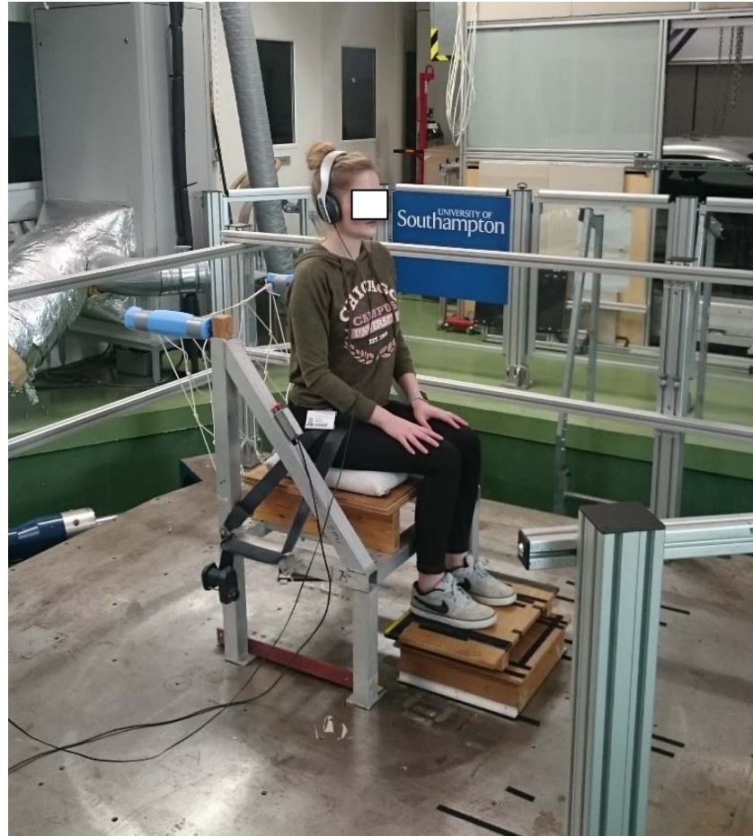
Figure 7.2 Experimental setup on the 6-axis vibration simulator.
