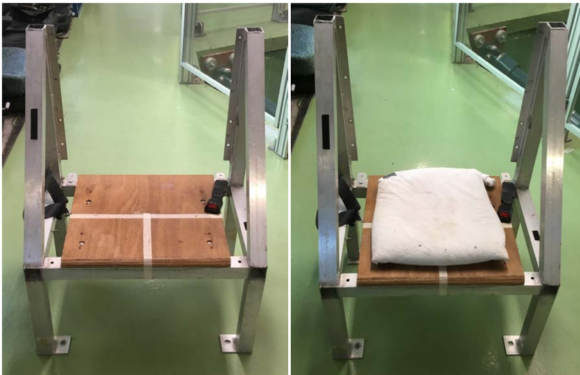
Figure 3.5 Rigid seat used in experiments 3 and 4 with and without the beanbag
