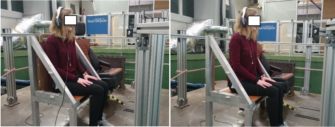
Figure 4.3 Experimental setup on the 6-axis simulator with backrest (left) and without backrest (right).
