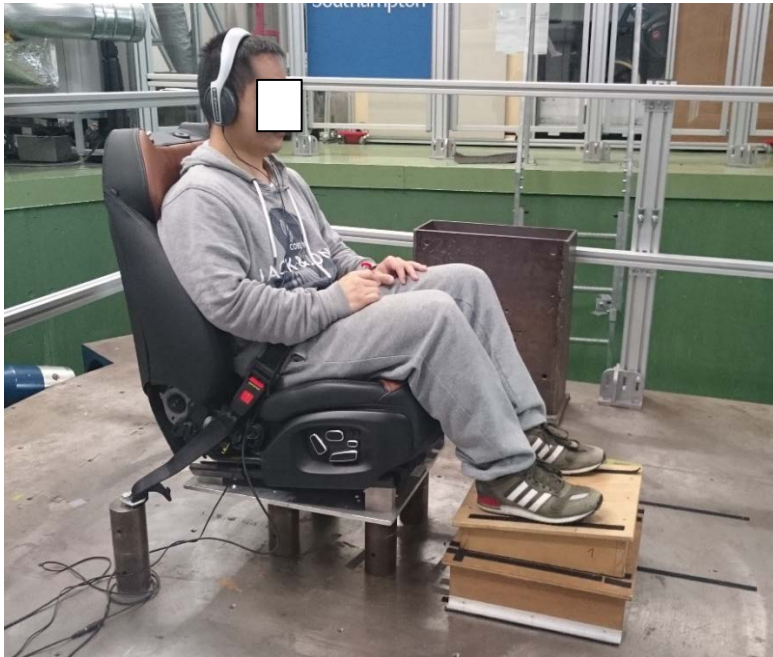
Figure 5.4 Experimental setup on the 6-axis simulator
