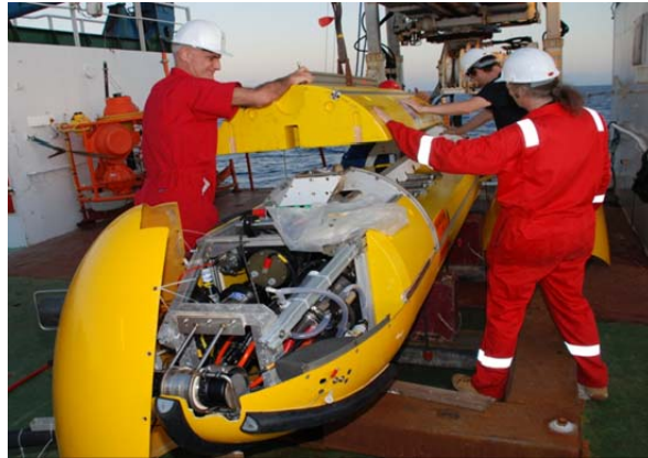
Figure 2.6: Getting Autosub6000 ready for a mission at the Cayman Rise. The removed front panel gives a clear view on the mechanical scanning sonar. Photo provided by the National Oceanography Centre, reproduced with permission.
