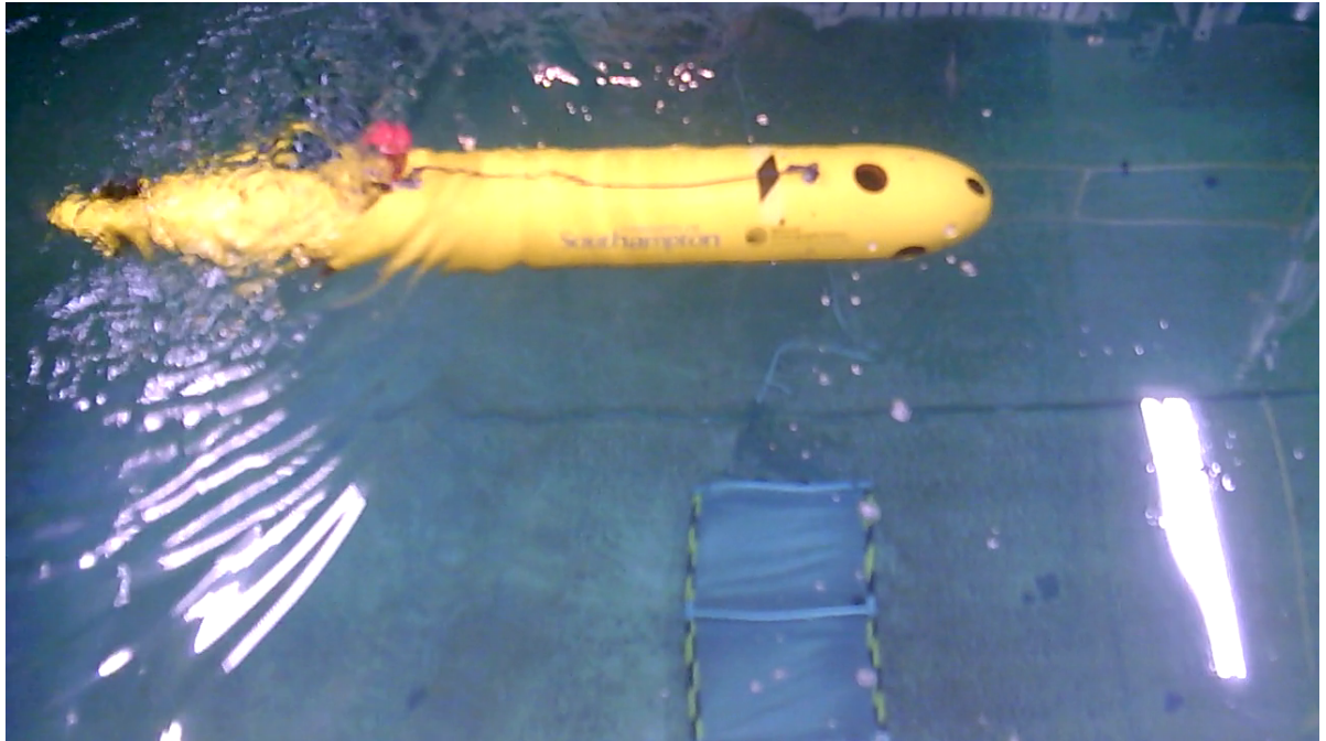
Figure C.1: Delphin2 in towing tank with a step obstacle made from metal shelf and bubble wrap.
