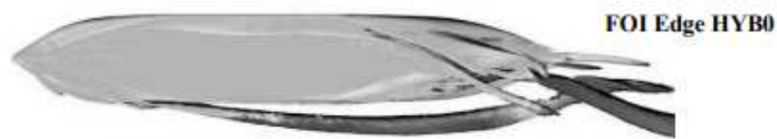
FIGURE 2.7: Vortical Structures from KVLCC2 Abdel-Maksoud et al. (2015)
