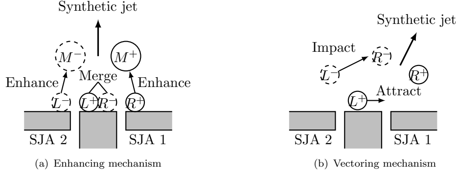
Figure 2: Interaction between synthetic jets, redrawn from Luo and Xia (2008). Synthetic jets in absence of a phase difference, leading to an enhanced merged jet (a) and synthetic jets with a phase difference, leading to a vectored jet (b).
