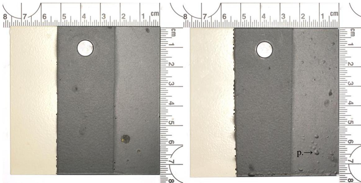
Figure 99: Coating system 5, coupon 286 (left) exposed to temperate inland site after 84 days with addition of 1 mL 0.03 wt. %  $\text{H}_2\text{O}_2$  solution twice per week, coupon 293 (right) exposed to temperate inland site for 84 days with addition of 1 mL 3 wt. %  $\text{H}_2\text{O}_2$  solution twice per week.
