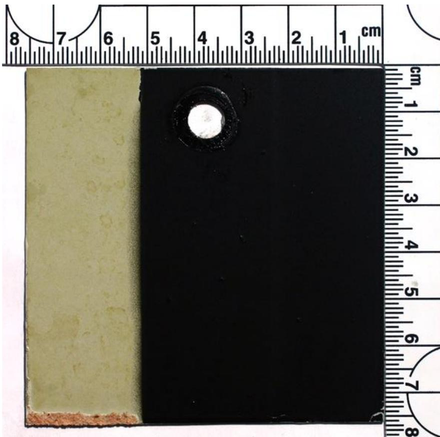
Figure 87: Post exposure image of Coating System 6 (Coupon #316) applied to AA7075-T6 exposed for 168 days to the temperate inland field exposure.
