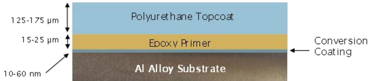
Figure 1: Military aerospace coating schematic.
