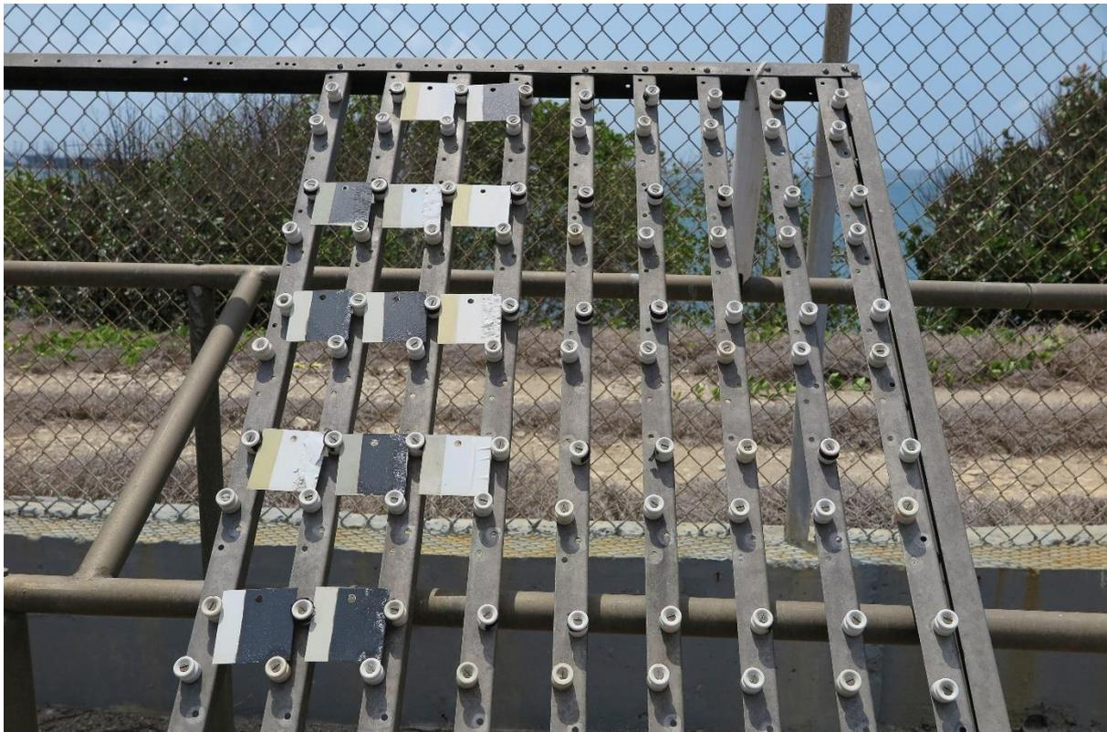
Figure 23: Tropical coastal exposure site at 336 days exposure.
