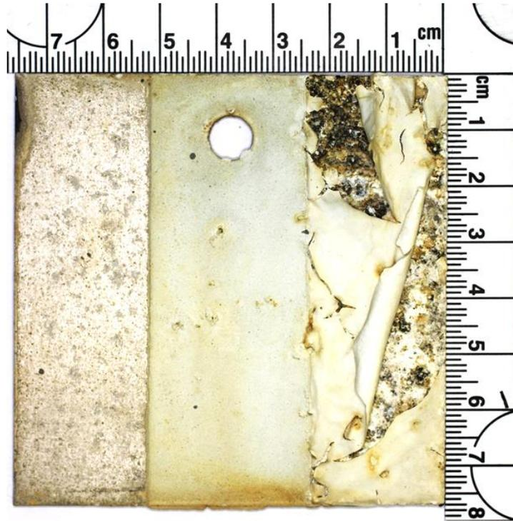
Figure 71: Coating System 1 in AA2024-T3 exposed to the tropical coastal site for 504 days (Coupon #58).
