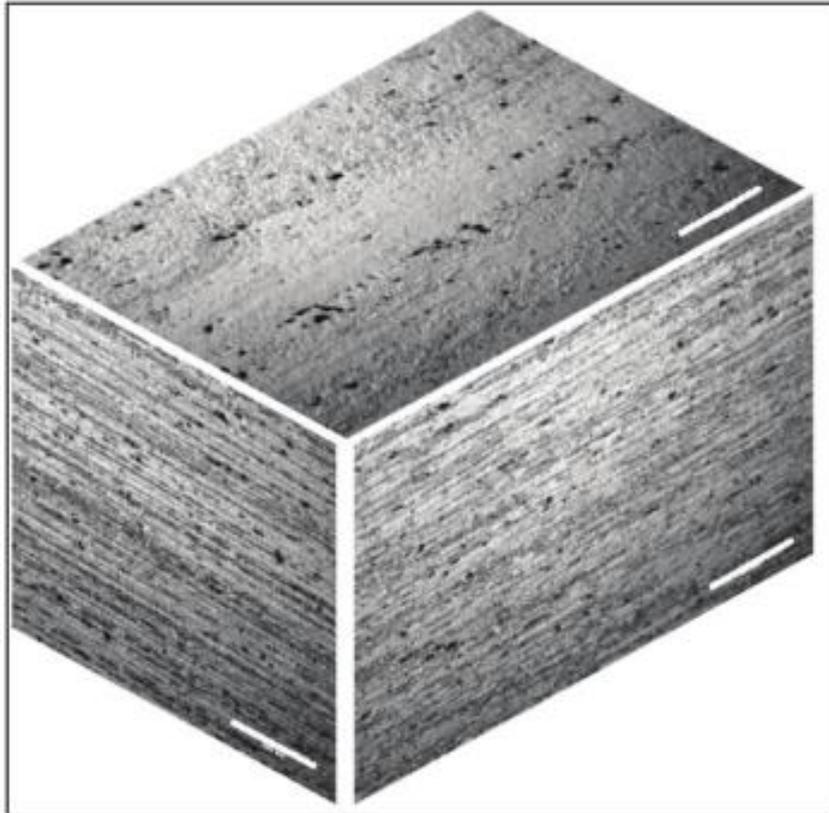
Figure 5: Microstructure of AA7075-T6, scale bar is a length of 100  $\mu\text{m}$  [5].
