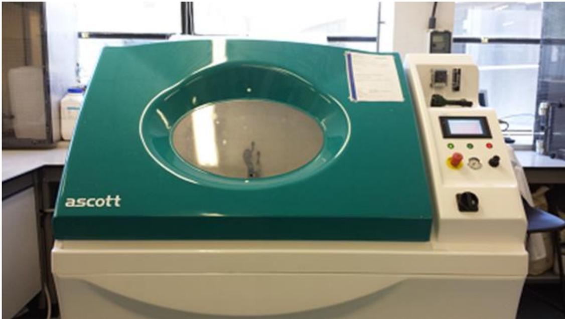
Figure 51: University of Southampton cyclic corrosion chamber.
