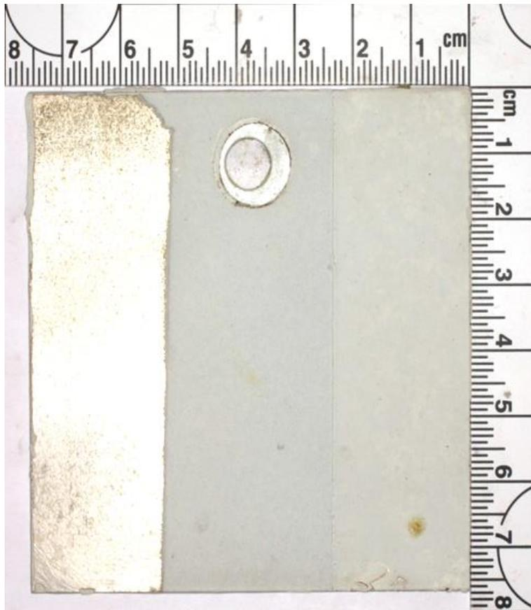
Figure 81: Post exposure image of Coating System 1 (Coupon #62) applied to AA7075-T6 exposed for 504 days to the temperate inland field exposure.
