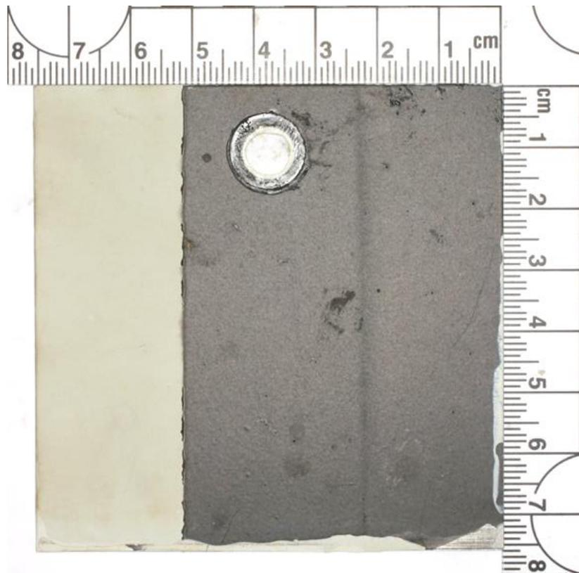
Figure 86: Post exposure image of Coating System 6 (Coupon #377) applied to AA2024-T3 exposed for 504 days to the temperate inland field exposure.
