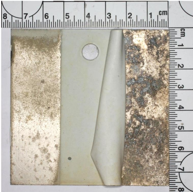
Figure 61: Coating system 1 on AA7075-T6 exposed to tropical coastal natural exposure for 420 days.
