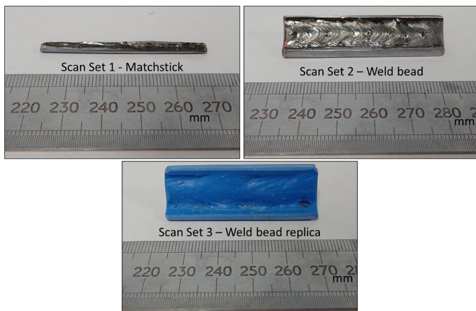
Figure 3.15 Photographs taken of a specimen from each of the three scan sets.
