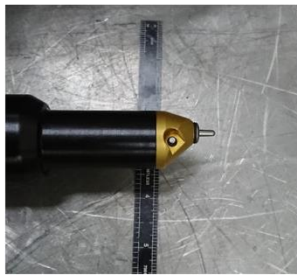
Figure 4.10 Images of the SONATS NOMAD UNP System and the result of peening on a welded specimen.
