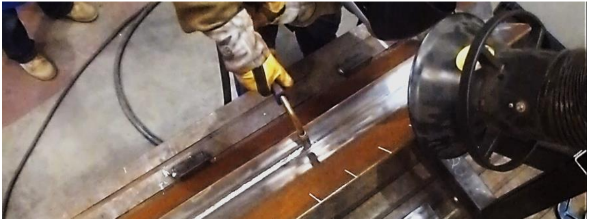
Figure 3.11 Manual MAG welder position before arc generation. From [9].
