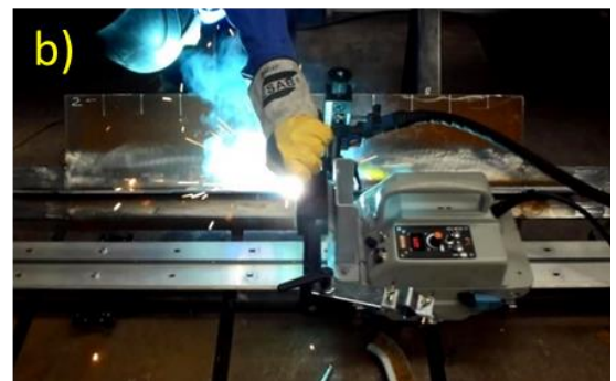
Figure 3.12 Semi-automated MAG welding – a) Arc-position; b) operator adjustment. From [9]
