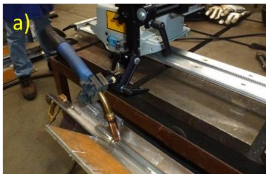
Figure 3.12 Semi-automated MAG welding – a) Arc-position; b) operator adjustment. From [9]
