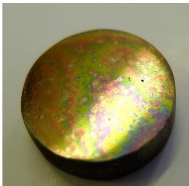
Figure 6.35 – Iridescent PoDA coating formed from a solution of 2 mg mL -1 dopamine in 0.1M phosphate buffer containing a 0.5:1 molar ratio of p -Benzoquinone to dopamine at 25°C: the S275 steel disc is 15 mm in diameter
