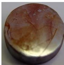
Figure 6.5 - Coating produced from a 3:1 ratio of \text{Na}_2\text{MoO}_4 to dopamine using a 2 \text{ mg mL}^{-1} dopamine in 0.1M phosphate buffer solution and a 25^\circ\text{C} deposition temperature: the S275 steel disc is 15 mm in diameter. The EIS is carried out in 3.5%NaCl.
