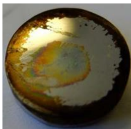
Figure 6.4 - Coating produced from a 3:1 ratio of \text{KMnO}_4 to dopamine using a 2 \text{ mg mL}^{-1} dopamine in 0.1M phosphate buffer solution and a 25^\circ\text{C} deposition temperature: the S275 steel disc is 15 mm in diameter. The EIS is carried out in 3.5%NaCl.
