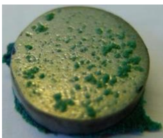
Figure 6.3 - Precipitation of copper (II) phosphate from a 2 \text{ mg mL}^{-1} dopamine in 0.1\text{M} phosphate buffer solution containing a 3:1 molar ratio of \text{Cu}(\text{OAc})_2 to dopamine at 25^\circ\text{C} : the S275 steel disc is 15 mm in diameter
