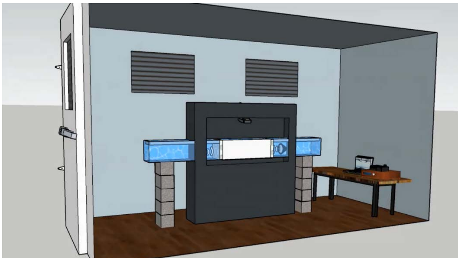
Figure 3.7: Section view schematic of still-water flume set-up within acoustically isolated chamber.
