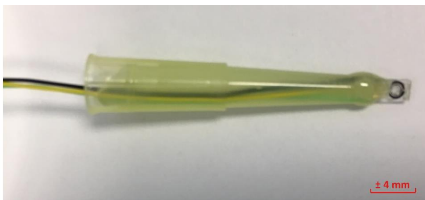
Figure 3.3 – Encapsulated sensor device prior to experimental use of sensor Type-C. The sensor and wires have been pulled through a pipette tip which is then filled with epoxy.
