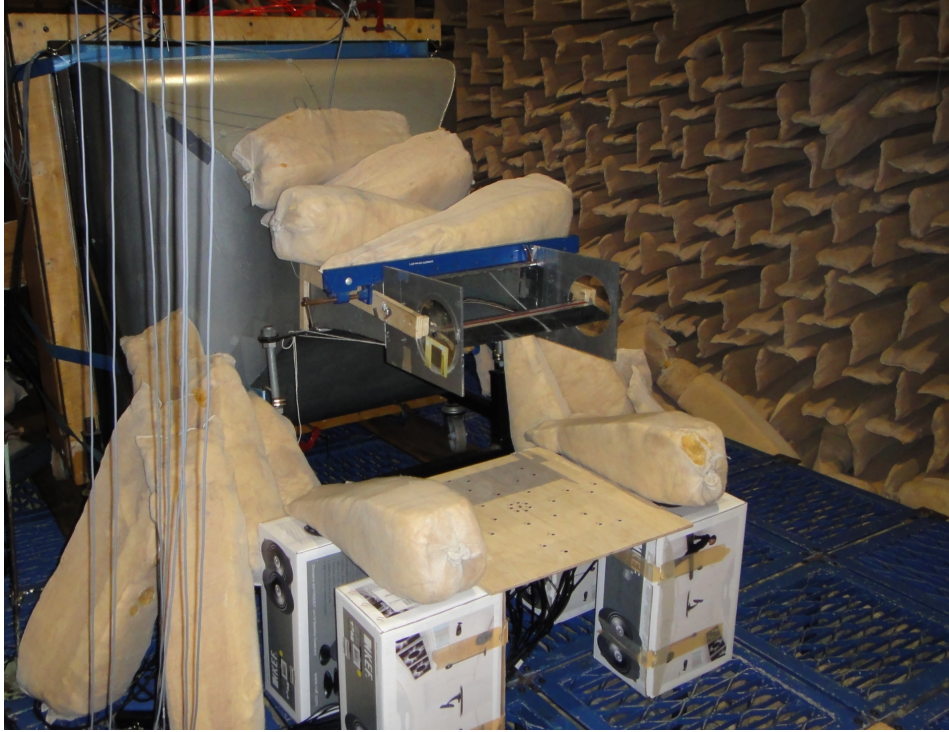
Figure 5.1: Photograph of the experimental setup; the aerofoil is attached to the wind tunnel nozzle, and the near-field microphone array is visible underneath it.
