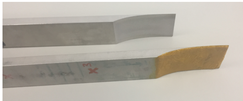
FIGURE 2.12: A picture of the ABH that was used in the experimental study, with and without damping.
