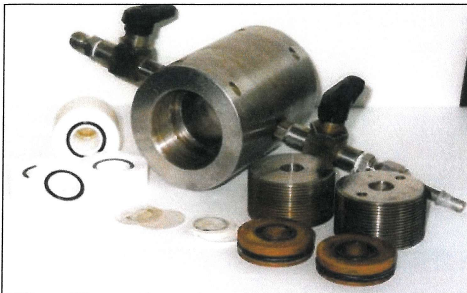
Figure 3-2: Picture of transmission EXAFS pressure cell showing cell body, boron nitride disks, and spacers.
