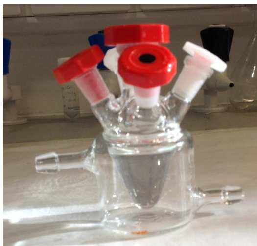
Figure 2.1 Picture of a 15 ml water-jacketed glass cell with five necks.
