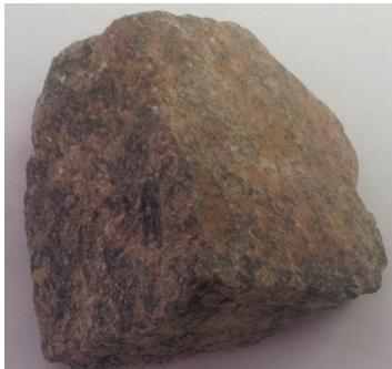
Figure 1.2: Ballast particle
