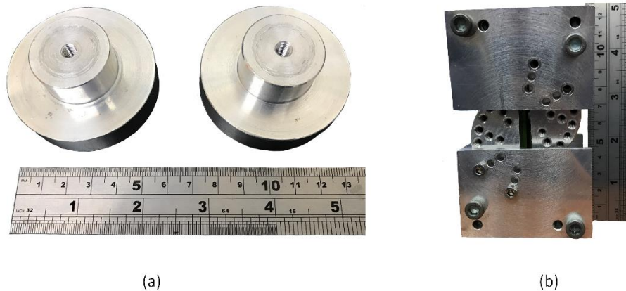
Figure 3.25: Custom-made (a) compression platens and (b) shear platens
