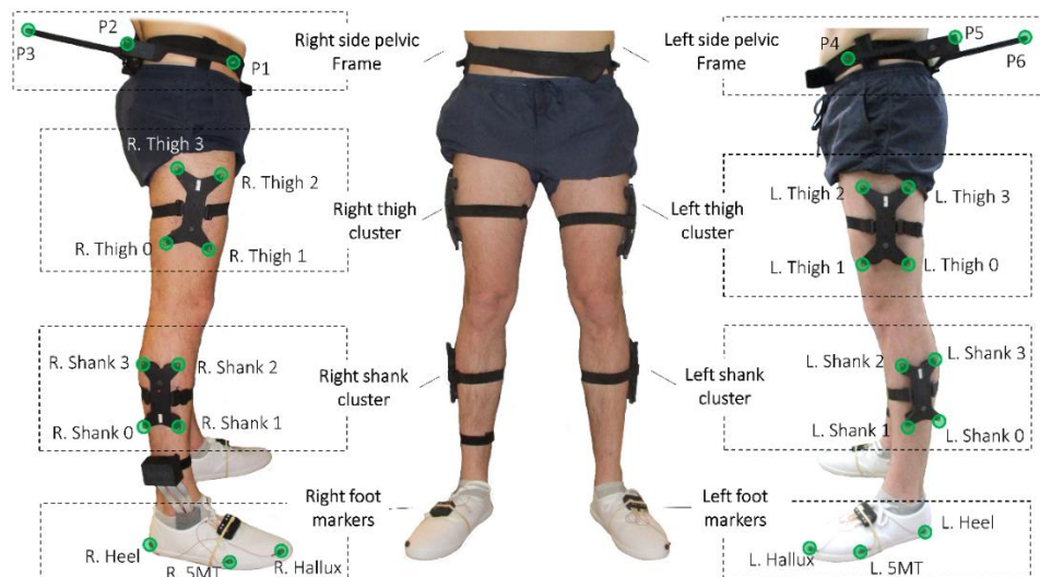
Figure 3.6: Real marker placement on the able-bodied participant.
