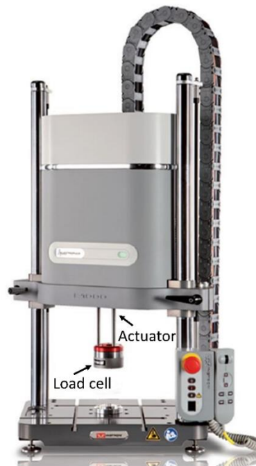
Figure 3.24: A photo showing the Instron ElectroPuls™ E1000 material test machine[229].
