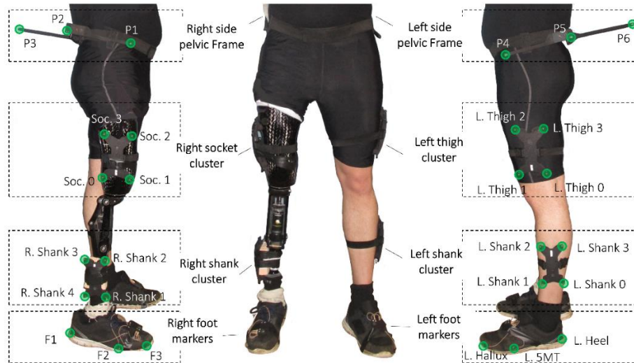
Figure 3.7: Real marker placement on the knee disarticulation amputee.
