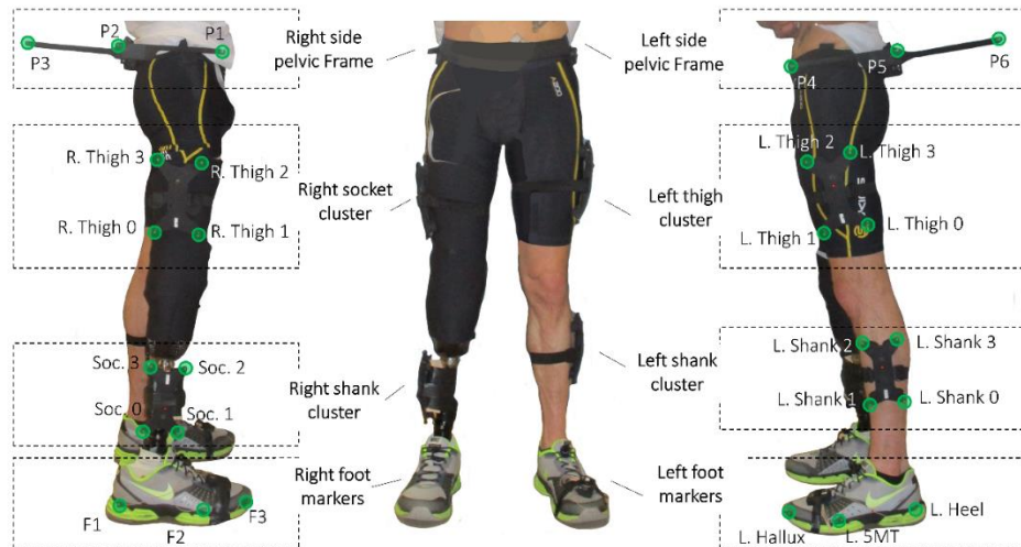
Figure 3.8: Real marker placement on the trans-tibial amputee.
