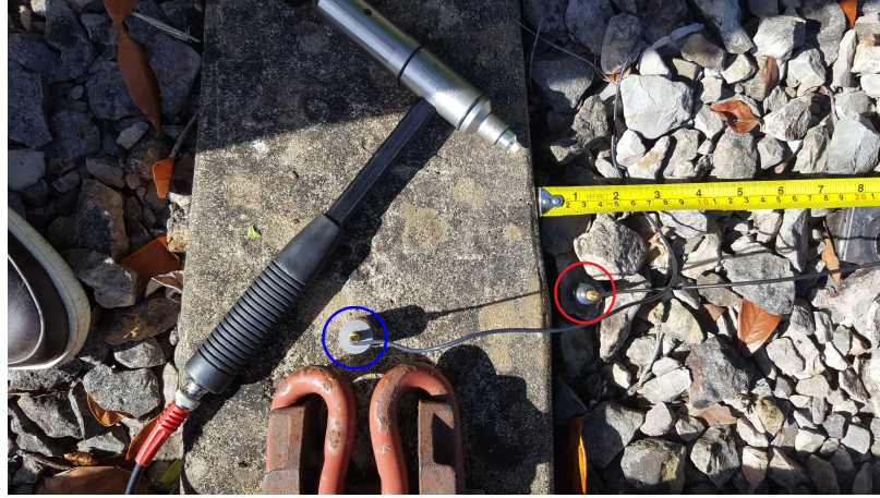
Figure 5.13. Measurement setup for the track vibration test: (a) top view of the track and the accelerometers and (b) the actual setup; ○ accelerometer on the sleeper, ○ accelerometer on the ballast
