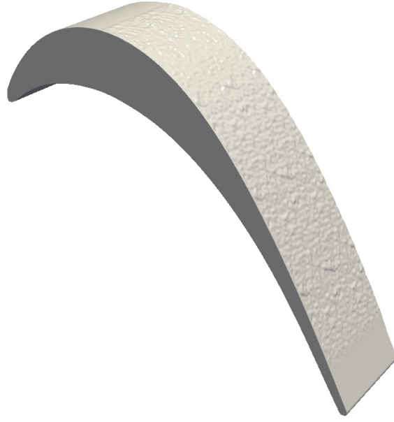
FIGURE 5.5: T106A turbine blade with multiple patches mapped onto the blade's suction surface by means of a rotation matrix.
