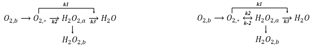
Figure 11. Example models for the ORR. On the left model suggested by Damjanovic et al. [70], on the right model proposed by Bagotskii et al. [26]. Subscript “a” means adsorbed on electrode surface, “b” means in bulk solution, “*” means in the vicinity of electrode surface.
