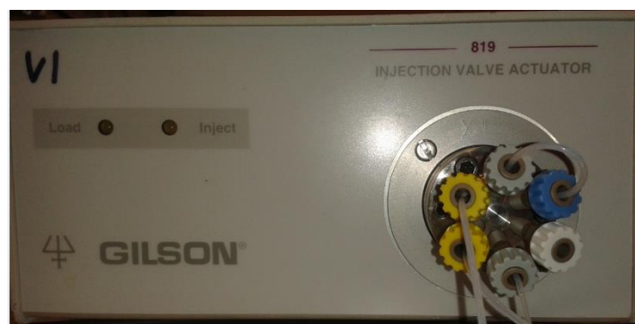
Figure 4.19: Gilson valve with its six connection points and two mode LEDs.
