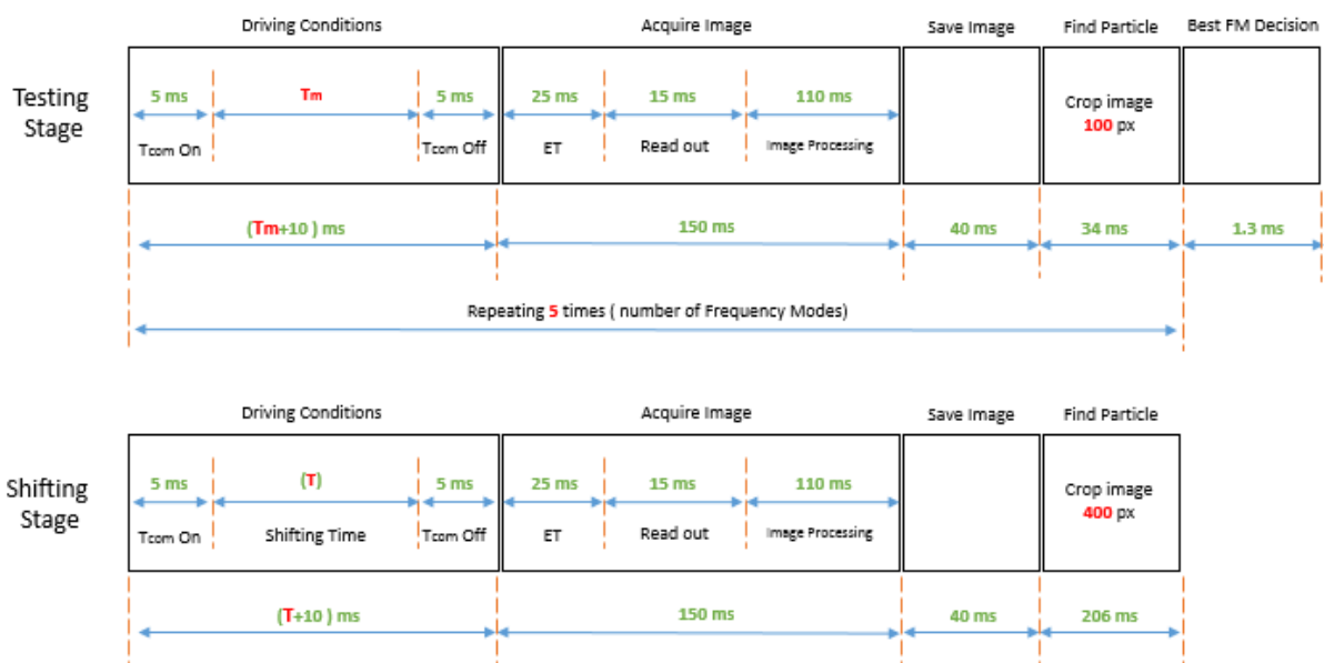
Figure 6.8: Sketch of steering system timings for both stages (testing and shifting) where T_m is the testing time and T is the shifting time. 1670 ms is the total typical testing time of 5 frequency modes with 100 ms pulse length each. 1406 ms is the typical total shifting time with 1000 ms shifting time for one selected frequency mode.
