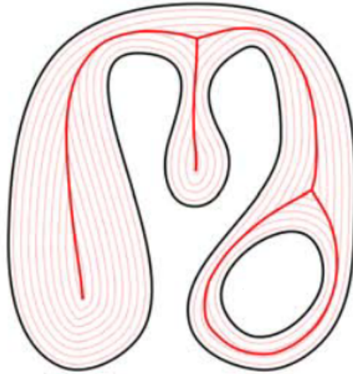
Figure 2.2: The medial axis grassfire (adapted from Tagliasacchi et al. (2016) ).
