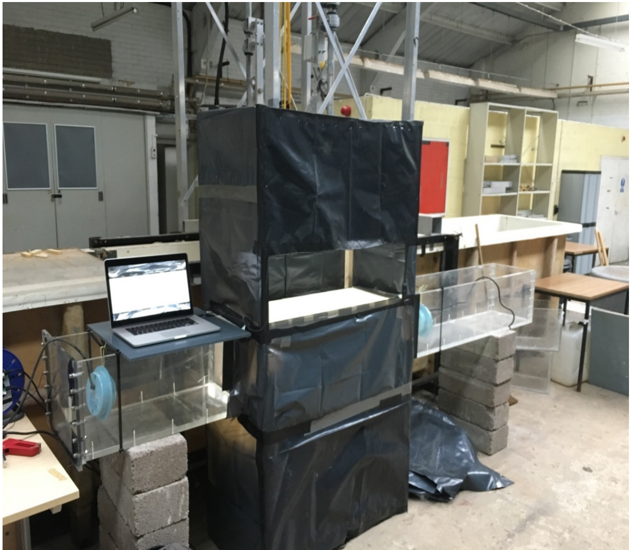
Figure 3.7 Experimental flume and black-out structure. The speakers (in blue) are also clearly visible outside of the experimental area. When trials are in progress there is an extra piece of black plastic which is secured over the visible gap.
