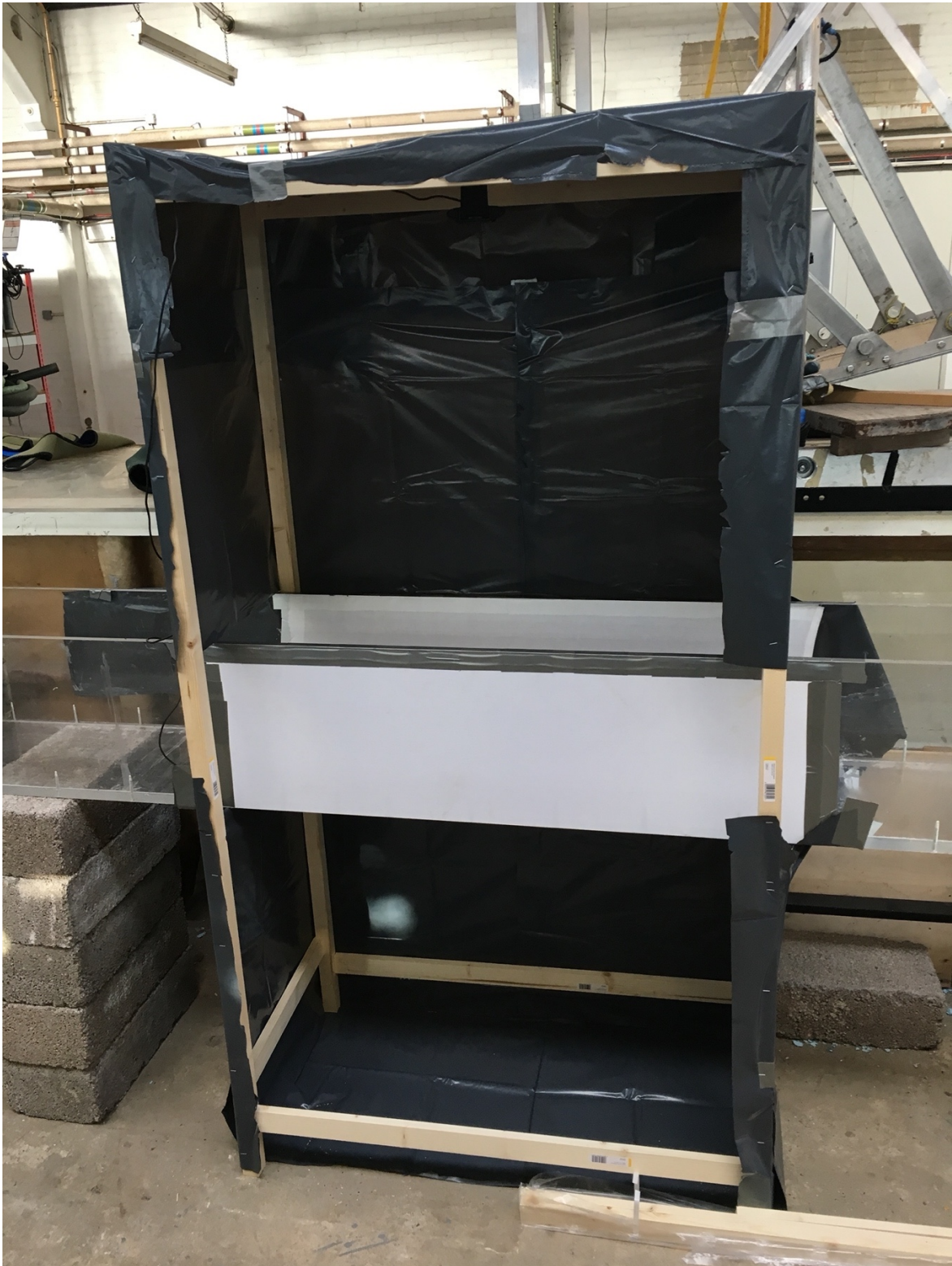
Figure 3.6 A photograph of the experimental area of the acrylic flume tank. Note the blackout structure encompassing this area and the white sheet material used to remove visual cues for fish and provide high contrast for video tracking. The space underneath the tank was used to place photographic lamps with large diffuser plates on.
