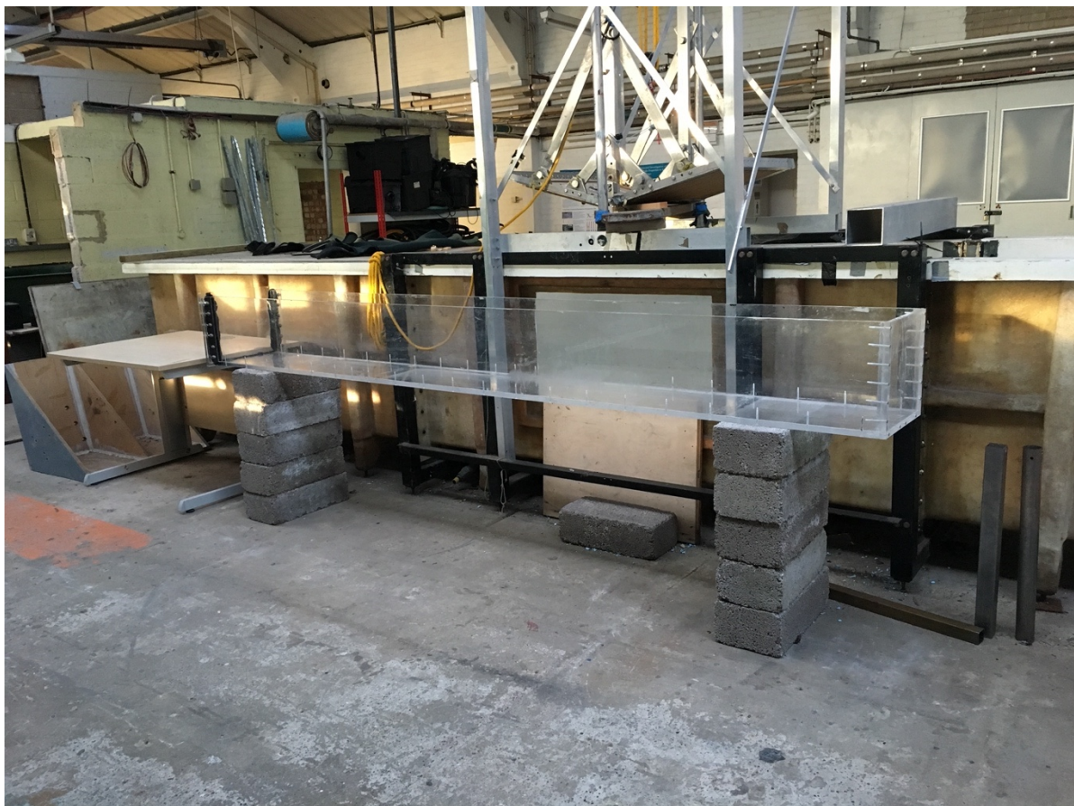
Figure 3.5 A photograph of the experimental flume tank used in the research detailed in this thesis. Note the transparent acrylic construction and the concrete-block plinths the tank is mounted on.
