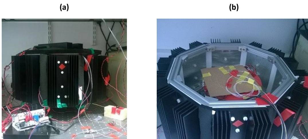
Figure 6-7 (a) Outside look and (b) inside look of the thermal chamber with 10 Peltier modules.
