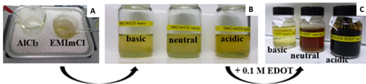
Figure 6: (A) Synthesis of EMImCl- \text{AlCl}_3 ionic liquid in a cooling bath. (B) Resulting Lewis basic, neutral and acidic solution. (C) Addition of 0.1 \text{ mol dm}^{-3} EDOT and resulting Lewis basic, neutral and acidic solutions for electropolymerisation. 48
