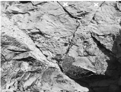
Figure 2.13 An example of fractured chalk bedrock (Lord et al. 2002): A) Offsets on conjugate faults (marked X) in the Newhaven Chalk Formation, Sussex; B) Frequency of horizontal joints predominates over the vertical ones, trial pit, A27 Brighton Bypass, The Upper Newhaven Chalk.
