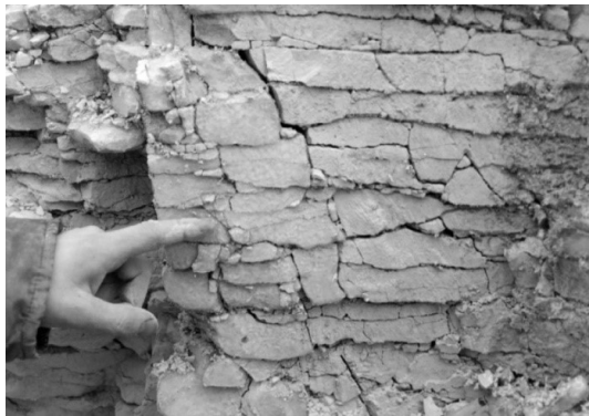
Figure 2.13 An example of fractured chalk bedrock (Lord et al. 2002): A) Offsets on conjugate faults (marked X) in the Newhaven Chalk Formation, Sussex; B) Frequency of horizontal joints predominates over the vertical ones, trial pit, A27 Brighton Bypass, The Upper Newhaven Chalk.
