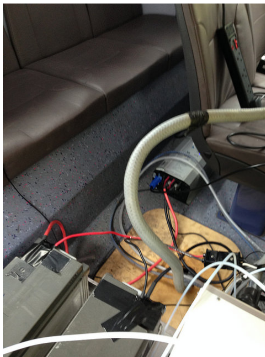
FIGURE 3.3: The in-cabin engine access panel was replaced with a custom panel allowing connections to the tailpipe attachment to be routed into the cabin whilst preventing engine noise and exhaust fumes from entering.
