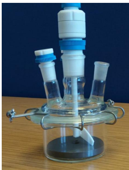
Figure 4.6. Custom glassware to accommodate silicon nitride discs.
