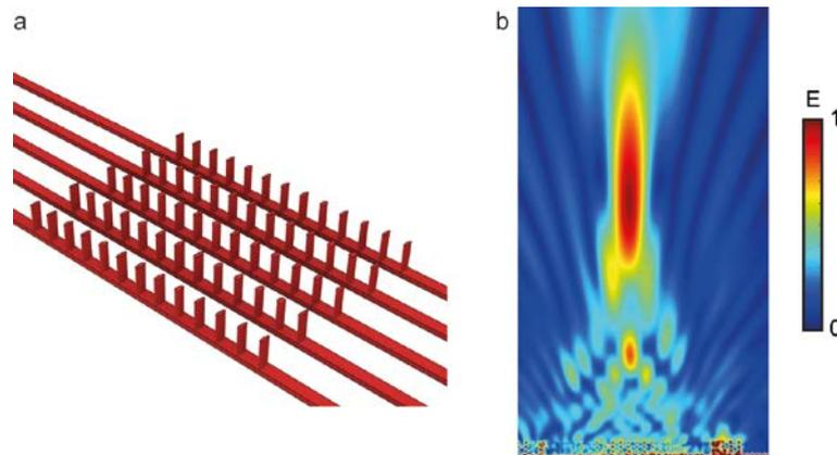
**Fig. 1:** Device schematic and light focusing. (a) A schematic of silicon metasurface comprising an array of silicon pillars located on top of parallel silicon waveguides. (b) A specific pillar configuration can focus light at a specific spot in the free space. The electric field profile corresponds to an area of  $20\ \mu\text{m}$  (width)  $\times$   $40\ \mu\text{m}$  (height).
