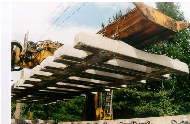
Figure 3.5: Modified Ladder track or Frame sleeper track (Riessberger, 2001)
