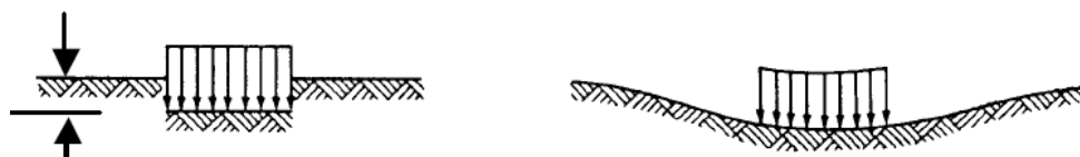
Figure 4.14: FEM foundation vs FDM foundation model
