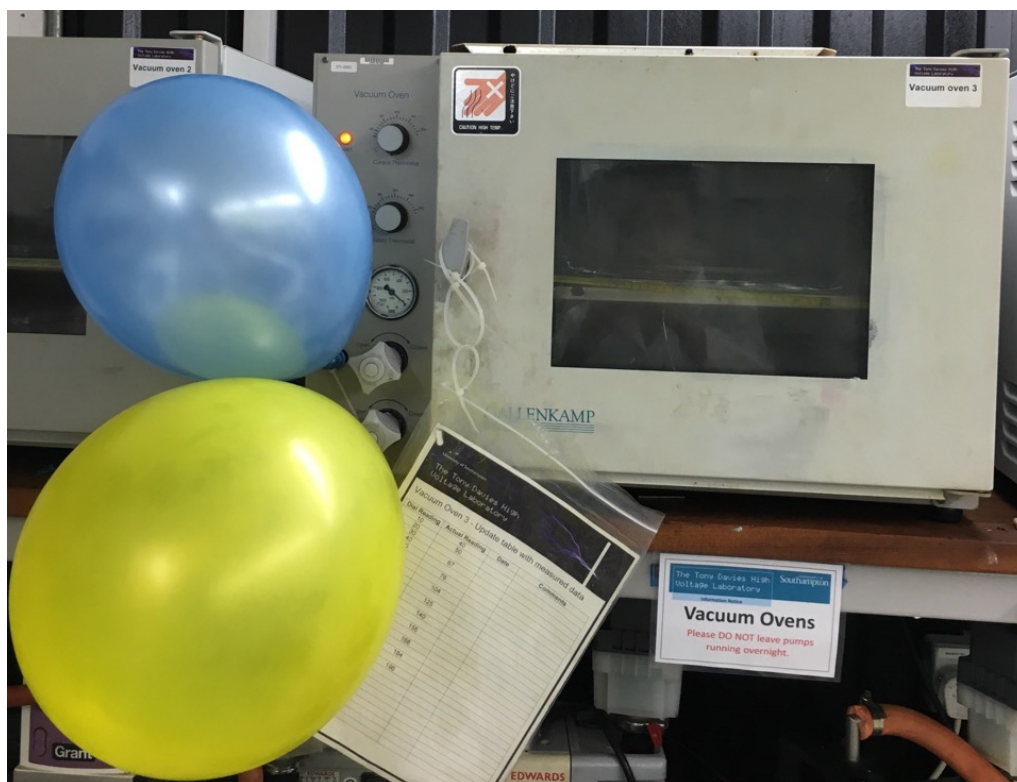
Figure 3.1: Thermal ageing installation in nitrogen in vacuum oven.
