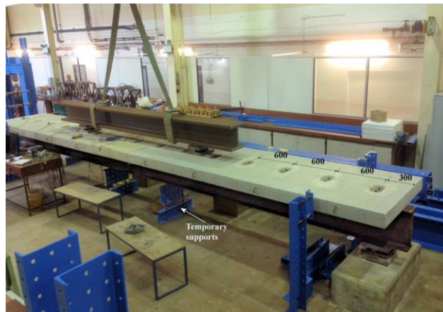
Figure 5.2: Experimental testing of a steel-concrete composite beam with FBSC [36].
