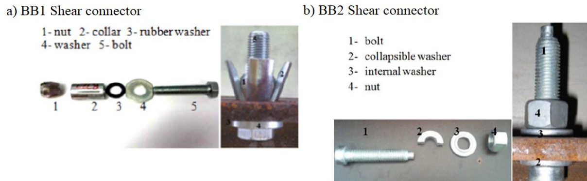
Figure 2.17: Blind bolts used as shear connectors – Pathirana et al. [28].
