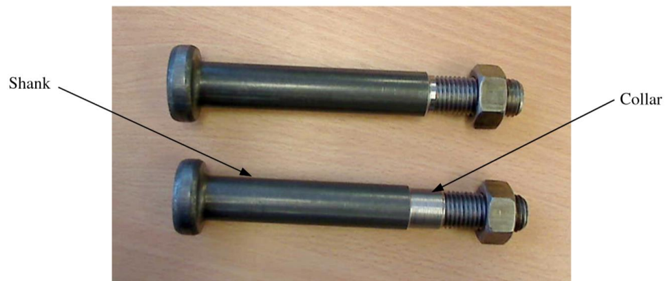
Figure 2.10: Demountable shear connector manufactured from standard headed studs – Lam and Saveri [20].
