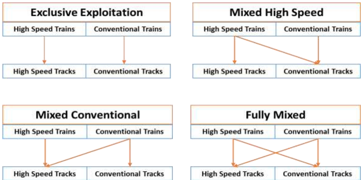
Figure 2-1: High-speed degrees of separation. (Source: Rutzen and Walton, 2011; de Rus, 2012a, 2012b)
