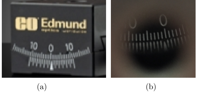
Figure 17: Goniometer vernier with a pitch angle resolution of 0.1^\circ in (a) and an image of the vernier used to record the angle during a test in (b).
