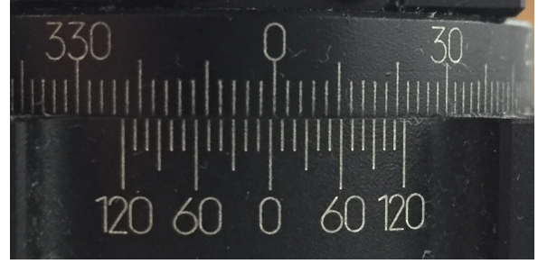
Figure 18: Rotary stage vernier with a yaw angle resolution of 0.17^\circ .
