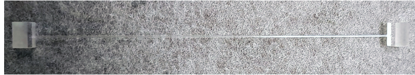
FIGURE 6.3: The end-capped fibre-rod.
