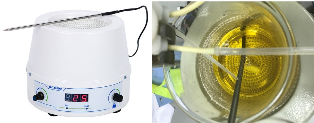
Figure B3. Heating mantle and thermocouple used to heat up the oil. Image on the left is for illustrative purposes only.
