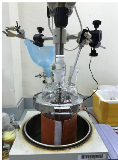
Figure A7. Installing the reactor system with the impeller clamped to the overhead motor.
