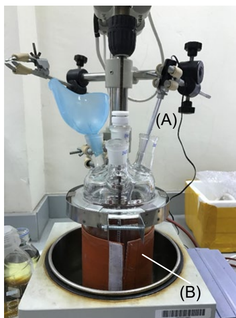
Figure 4-88. The glass reactor setup with the heating mechanism, (a) Thermocouple, (b) Heating jacket.
