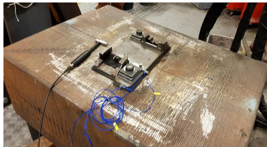
Figure 5-9 View of the rig setup for the measurement setup of the two-stage baseplate.
