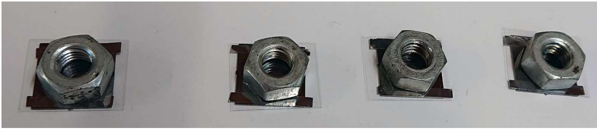
Figure 28: polished samples with stainless steel spacer shims, coating, coverglass and 10.3g weight (nut)
