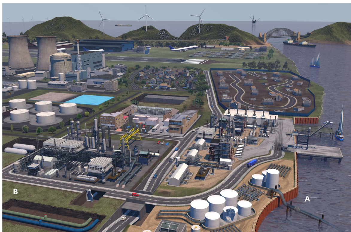
Figure 2: Schematic of some generalised uses of coatings, including unsaturated polyesters. Zone A: Marine. Unsaturated polyesters are commonly used around marine areas including retaining walls, oil rigs, splash-zone of riser piles or jetty piles, tank exteriors, and some ship applications. Unsaturated polyesters can be used for water inlet/outlet pipes and tanks or reservoirs of water. However, tanks containing chemicals will generally require more chemical resistance and be coated with several layers of vinyl esters. Zone B: Underground. Epoxies make great protective coatings, but their tendency to chalk when exposed to light means they are best suited for underground applications (or under a UV resistant topcoat).
