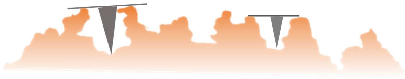
Figure 17: schematic of a profile measurement by profilometer. Several measurements of peaks to valleys are taken and the average is reported.
