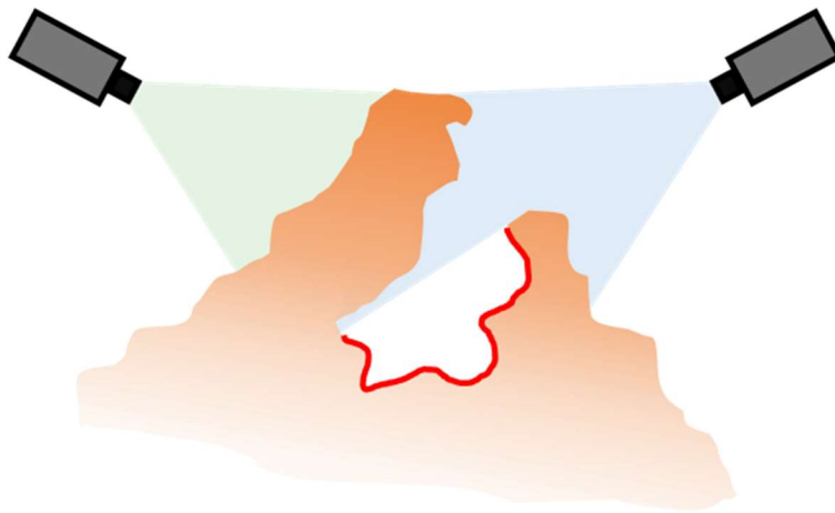
Figure 21: Schematic of problematic crag in a sample for 3D microscopy. In this case, the cameras (in black) cannot “see” the surface highlighted in red as it is blocked from view by the nearby peaks.
