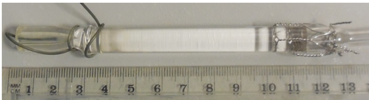
Figure 68: Silica calibration preform used in vertical scanning calibration measurements.
