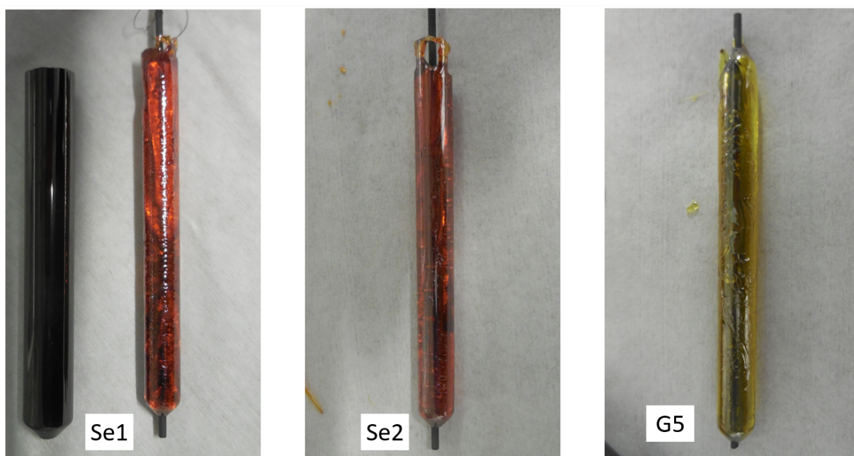
Figure 52: Embedding 2 mm graphite rods in GLSSe20% by casting around. Se1, first test with graphite, GLSSe20% cast in a 600 °C mould. Length-wise cracks are visible. Se2, repeat in a 650 °C mould. Appeared intact at the time, but spontaneously cracked after being taken out. G5, repeat of Se2 using GLSO instead, to ensure the reproducibility of the success achieved with GLSO. Cast remained intact indefinitely.
