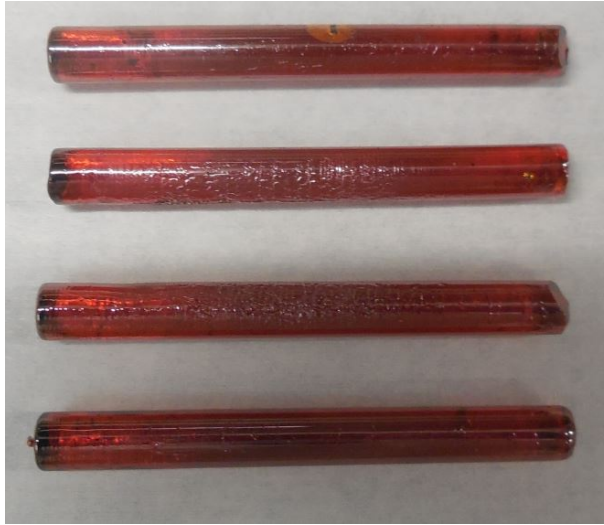
Figure 48: GLSSe20% glass cast into 300 °C vitreous carbon moulds, fabricated to later be drawn into canes using the fibre drawing tower.
