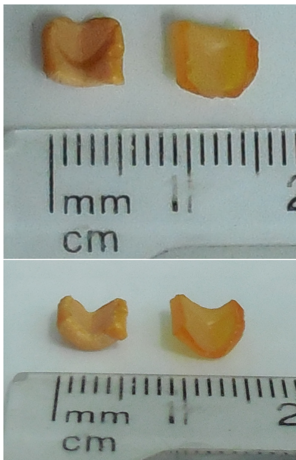
Figure 34: Sample remains of TMA three-point bending: crystallized (LD1900) on the left, non-crystallized (LD1899) on the right.
