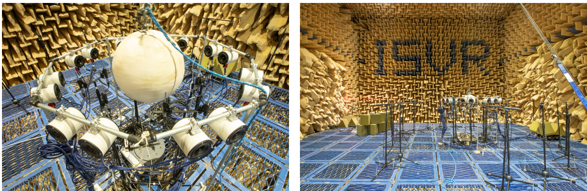
Figure 2.3: Images of the experimental setup, showing the rigid sphere, the loudspeaker array, and the far-field microphone array.
